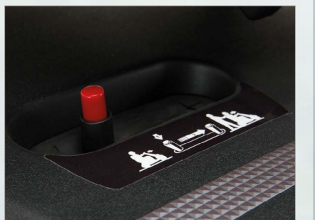
Two-step disengaging lever to prevent free-wheeling
